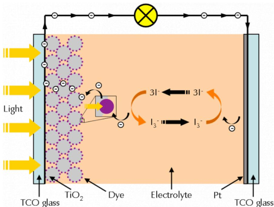
Figure 1. The structure of a dye-sensitized solar cell. From: Gamry.com.
